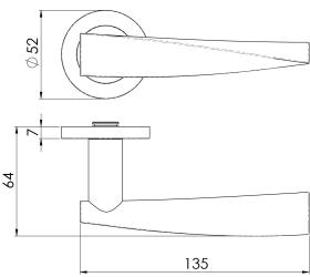
Lever on a concealed fix threaded rose. A stunning eye catching design. The lever has an angular downward twist making it ergonomic in use as well as being extremely stylish. Part of the Steelworx range in grade 304 Stainless Steel.
