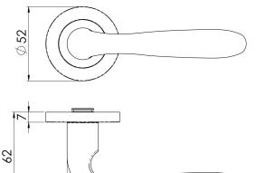
Lever on a concealed fix threaded rose. The lever is slightly bulbous almost torpedo shaped making it very comfortable to grip. Part of the Steelworx range in grade 304 Stainless Steel. Comes with a 10 year mechanical guarantee and is Fire door rated.
