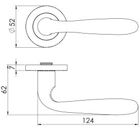
Lever on a concealed fix threaded rose. The lever is slightly bulbous almost torpedo shaped making it very comfortable to grip. Part of the Steelworx range in grade 304 Stainless Steel. Comes with a 10 year mechanical guarantee and is Fire door rated.
