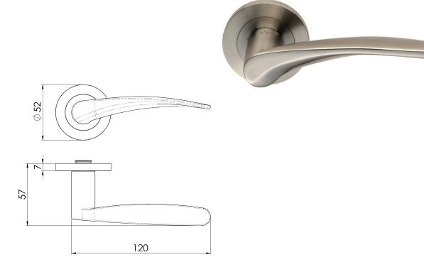
Lever on a concealed fix threaded rose. The lever is slightly curved with an angled forefront as a thumbgrip making it very comfortable to hold. Part of the Steelworx range in grade 304 Stainless Steel. Comes with a 10 year mechanical guarantee and is Fire door rated.
