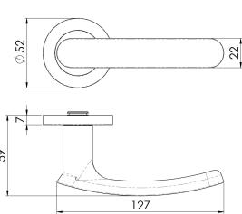
Lever on a concealed fix threaded rose. The bold face of the lever is slightly curved with rounded ends for safety. Part of the Steelworx range in grade 304 Stainless Steel. Comes with a 10 year mechanical guarantee and is Fire door rated.
