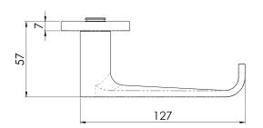
Lever on a concealed fix threaded rose. A straight bold faced lever with a rounded return to door end for safety. Part of the Steelworx range in grade 304 Stainless Steel. Comes with a 10 year mechanical guarantee and is Fire door rated.
