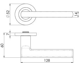
Lever on a concealed fix threaded rose. A slender straight lever with an elliptical shape. The smooth rounded edges gives it a minimalist look. Part of the Steelworx range in grade 304 Stainless Steel.
