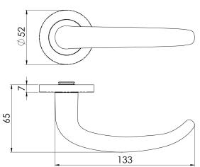
Lever on a concealed fix threaded rose. A slender straight rounded lever with a gentle inward curve at the end. Part of the Steelworx range in grade 304 Stainless Steel. Comes with a 10 year mechanical guarantee and is Fire door rated.
