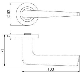
Lever on a concealed fix threaded rose. A chunky flat bar lever tapering towards the end. Part of the Steelworx range in grade 304 Stainless Steel. Comes with a 10 year mechanical guarantee and is Fire door rated.
