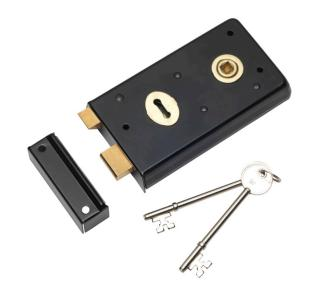
Traditional style Rim Lock generally for use on internal doors, gates, shed doors. Certified to BS EN 12209. This lock carries a 5 year mechanical guarantee. It has been CE and Certifire tested.
