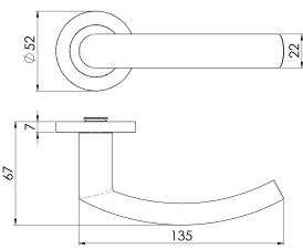
Lever on a concealed fix threaded rose. The rounded lever is slightly curved making for a comfortable grip. Part of the Steelworx range in grade 304 Stainless Steel. Certified to BS EN 1906.
