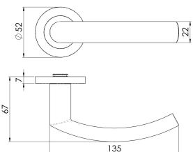
Lever on a concealed fix threaded rose. The rounded lever is slightly curved making for a comfortable grip. Part of the Steelworx range in grade 304 Stainless Steel. Certified to BS EN 1906.
