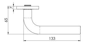
Lever on a concealed fix threaded rose. A straight round bar lever. Part of the Steelworx range in grade 304 Stainless Steel. Comes with a 10 year mechanical guarantee and is Fire door rated.
