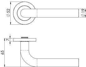
Lever on a concealed fix threaded rose. A straight round bar lever. Part of the Steelworx range in grade 304 Stainless Steel. Comes with a 10 year mechanical guarantee and is Fire door rated.
