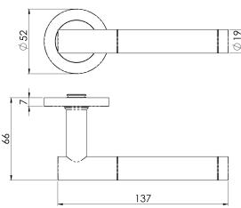
Lever on a concealed fix threaded rose. A round bar lever with a ringed design. Part of the Steelworx range in grade 304 Stainless Steel. Comes with a 10 year mechanical guarantee and is Fire door rated.
