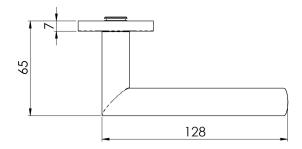
Lever on a concealed fix threaded rose. A round bar lever with an ergonomic high curve design. Part of the Steelworx range in grade 304 Stainless Steel. Certified to BS EN 1906.
