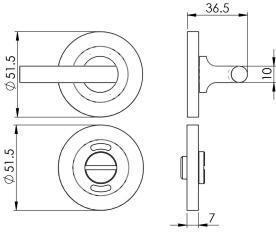
A modern style turn and release with or without indicator to match the SWL Levers. A long cylindrical turn for easy operation with a coin release on the other side in case of emergency access and a coloured segment to signal if engaged or vacant. Part of the Steelworx range in grade 304 Stainless Steel. Comes with a 10 year mechanical guarantee.
