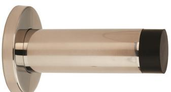
3 Inch and 4 Inch Wall Mounted Door Stops. Cylindrical door stop with rubber buffer on a round rose. The base rose unscrews allowing it to be fixed to the wall or skirting board. The door stop main body is then screwed back on for neat concealed fix.
