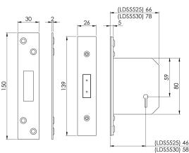
Easi-T Lever 5 Lever Deadlock in 64mm or 76mm options. Certified to BS EN 12209 Lock used as a matter of course by the national house builders. This lock provides a good degree of security and carries a 10 year mechanical guarantee. It has been CE and Certifire tested.
