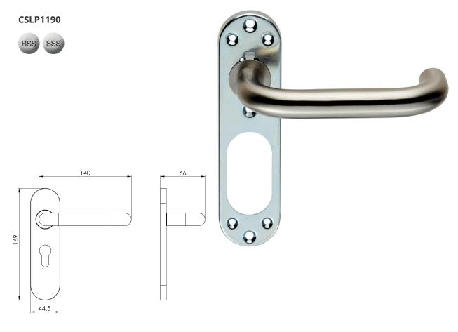
Optional Lever Templates. Straight Lever on Inner Plate and Safety Lever on Inner Plate. A multi function handle template which serves as a base for alternative covers making this a very useful and flexible product. Various covers can be fitted over the template thus converting it into a lock, latch or bathroom assembly as required.
