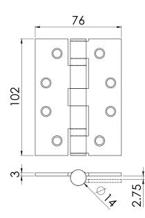
Grade 13 Ball Bearing Hinge, Square or Radius options. (Max Load 120kg). The most popular type of door hinge on the market today. They have a CE mark and are Certifire tested.
