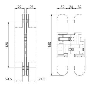
A concealed heavy duty hinge for unrebated, flush faced quality timber doors. Has removable cover plates to conceal the adjustment screws. Comes with a 10 year mechanical guarantee.
