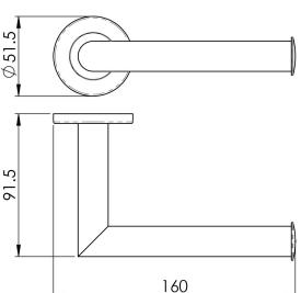
A simple toilet paper holder design. The mitred round bar is secured onto a concealed fix rose. DeLeau LX, a contemporary modern range of stylish bathroom fittings in Grade 316 Stainless Steel . Each component comes with fixing screws, wallplugs and concealed fixing plate.
