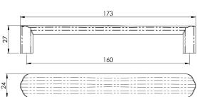
A straight handle with a unique ripple effect on the flat face extending around the rounded ends giving a positive grip in operation.
