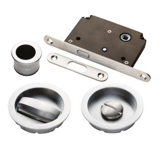
Sliding Door Set with WC Turn, Flush Pull and Lock. Sliding bathroom door set comprising of a turn and release, finger pull and a lock . The slim lock has a hook bolt which locates into a keep which is morticed into the frame. The thumb turn operates the lock mechanism and the coin release provides access in case of emergency.
