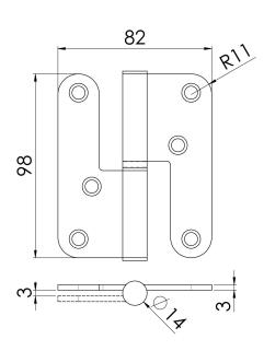
Grade 11 Lift Off (Journal Support) Hinge, Radius, Left or Right hand options. (Max Load 80kg). The special journal design gives maximum endurance with minimum maintenance requirements. The small bearing surface makes doors easy to open.
