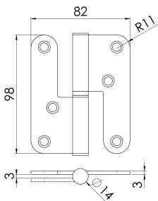
Grade 11 Lift Off (Journal Support) Hinge, Radius, Left or Right hand options. (Max Load 80kg). The special journal design gives maximum endurance with minimum maintenance requirements. The small bearing surface makes doors easy to open.
