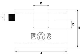
80mm Full clad armoured steel body. Keyed to Differ. Hardened steel plate shackle. Supplied with 3 brass keys.
