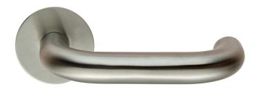
A substantial round bar return to door lever on a concealed fix ultra slim round unsprung rose. Part of the Steelworx SWB Blade range in grade 304 stainless Steel. The SWB Blade lever collection is a simple way to achieve a flush mounted appearance for door furniture without extensive routing. All that is required is preparation for the spindle hole and bolt fixing holes at 38mm c/c.
