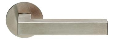
A substantial straight square bar lever on a concealed fix ultra slim round unsprung rose. Part of the Steelworx SWB Blade range in grade 304 stainless Steel. The SWB Blade lever collection is a simple way to achieve a flush mounted appearance for door furniture without extensive routing. All that is required is preparation for the spindle hole and bolt fixing holes at 38mm c/c.
