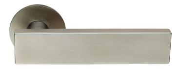
A substantial straight flat fronted rectangular lever on a concealed fix ultra slim round unsprung rose. Part of the Steelworx SWB Blade range in grade 304 stainless Steel. The SWB Blade lever collection is a simple way to achieve a flush mounted appearance for door furniture without extensive routing. All that is required is preparation for the spindle hole and bolt fixing holes at 38mm c/c.
