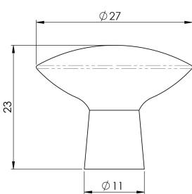
Disc shaped knob on a tapered stem reminiscent of a mushroom shape. This provides a comfortable grip and easy pull in operation.
