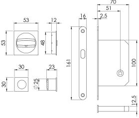
Sliding bathroom door set comprising of a turn and release, finger pull and a lock . The slim lock has a hook bolt which locates into a keep which is morticed into the frame. The thumb turn operates the lock mechanism. The flush fitting roses are sunk into the door and the coin release provides access in case of emergency.
