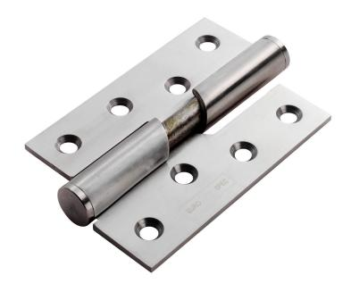
Rising Butt Hinge in Left or Right Hand options. Rising butt hinges are used to aid doors to self close in such environments as bathroom/toilet cubicles. As the door is opened the door rides up the spiral knuckle raising the door as it opens. When the door is released the weight of the door combined with the bevel on the hinged joint causes the door to close by itself in the majority of cases, although this action is not entirely reliable.
