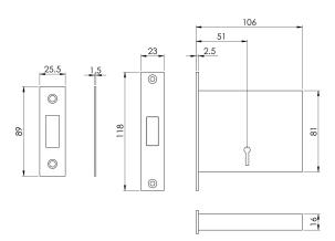
A 1-Lever mortice deadlock commonly specified and used by the London & South East Fire Brigade services, whereby the FB2 key will fit these FB2 locks so that access can be gained without damage to the door. Generally used on service riser doors in blocks of flats and other similar utility cupboards and rooms. Can also be used around the home or office as general deadlocks which all require the same keys..
