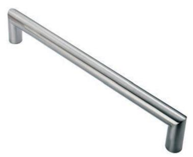
Mitred round bar cabinet pull handle. A robust 10mm Dia. round bar with either 96mm or 128mm c/c. Part of the Steelworx range in Grade 304 Stainless Steel.
