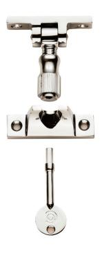
A traditional Brighton pattern sash window sprung fastener for narrow style window frames. Locking version. A classic method of fastening and locking sliding sash windows. To lock, pull the sprung toggle arm down and screw the knob into the keep.
