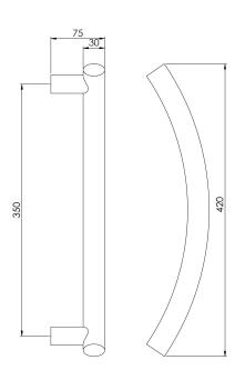
Curved T Pull Handle, a 30mm Dia. round bar sitting atop two inset pedestal stems with 350mm c/c. A classic tubular design making it suitable for many different environments, especially where a strong, hard wearing pull handle is required. Part of the Steelworx range in grade 316 Stainless Steel.
