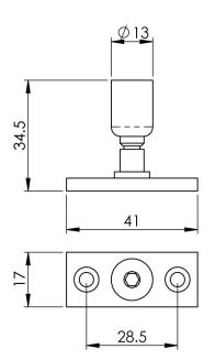
The locking casement stay pin makes it easy to lock your windows and add an extra layer of security to your home. Simply replace one of your standard stay pins with the locking pin. With the casement stay in the closed position screw the lock section of the pin assembly down with the key and remove the key. The simple and traditional design will fit the majority of casement stays on the UK market and can instantly provide extra security.
