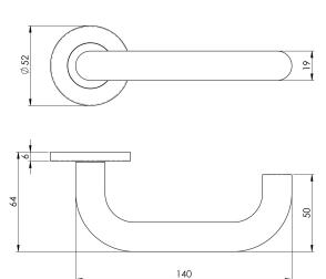
NERA Lever on concealed fix press on sprung round rose. Safety Lever, a 19mm round bar return to door lever. Ideal for public/office doors where a more ergonomic operation is a necessary requirement. Certified to BS8300 to meet the needs of disabled people.
