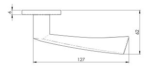
Breeze Lever on concealed fix press on sprung round rose. The lever has a flat wide top twisting slightly downward and with its ergonomic shape makes for a comfortable handle to operate. The CSL lever collection on a slim fit rose reflects the latest trends for subtle discreet fittings with ultra-modern styling and quality engineering. All levers are G304 grade with Grade 201 rose inners and a secure heso spindle fix, ensuring these products are of the highest calibre at competitive pricing.
