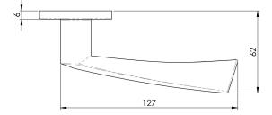
Breeze Lever on concealed fix press on sprung round rose. The lever has a flat wide top twisting slightly downward and with its ergonomic shape makes for a comfortable handle to operate. The CSL lever collection on a slim fit rose reflects the latest trends for subtle discreet fittings with ultra-modern styling and quality engineering. All levers are G304 grade with Grade 201 rose inners and a secure heso spindle fix, ensuring these products are of the highest calibre at competitive pricing.
