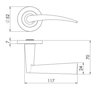
Volantes Lever on a concealed fix threaded slim rose. A slender flat bar handle, slightly arched, flaring marginally widthwise towards its end which accentuates its form in this modern design. The SWL lever collection on a slim 7mm rose reflects the latest trends for subtle discreet fittings with ultra-modern styling and quality engineering. All levers are G304 grade and come with a secure heso spindle fix, ensuring these products are of the highest calibre at competitive pricing.
