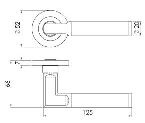
Carbon Fibre Lever on a concealed fix threaded slim rose. A straight round bar handle with a carbon fiber midsection. The neck stems from the rose in a rounded square section through a continuous right angle into the handle section, making this a truly outstanding lever and will appeal at many levels. The SWL lever collection on a slim 7mm rose reflects the latest trends for subtle discreet fittings with ultra-modern styling and quality engineering.
