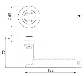
Soho Lever on a concealed fix threaded slim rose. A slender straight lever with an elliptical shape. The neck stems from the rose in a rounded square section through a continuous right angle blending into the tapering elliptical profile of the lever. The SWL lever collection on a slim 7mm rose reflects the latest trends for subtle discreet fittings with ultra-modern styling and quality engineering.
