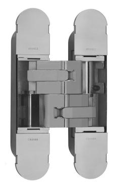
A concealed heavy duty hinge for unrebated, flush faced quality timber doors. Has removable cover plates to conceal the adjustment screws. Comes with a 10 year mechanical guarantee. Available in 6 different finishes, Suitable for doors from 35mm to 45mm thickness.
