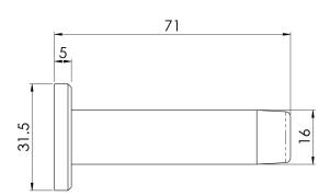
A 64mm rubber buffer tipped cylindrical door stop on a concealed fix rose.
