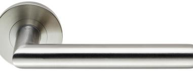
A Grade 4, Mitred straight round bar lever on a concealed fix screw on round rose with Abuse-resistant spindle. Part of the Steelworx range in Grade 316 Stainless Steel which offers the benefit of Anti Bacterial qualities associated with this grade. Will suit commercial and modern residential projects as they provide the quality and durability to cope within these environments. BS EN 1906 Rated 200.
