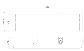
Overhead door closer EN2-5 by spring c/w backcheck c/w Fig 6 Bracket EN1154. Suitable for left and right hand application, Suitable for doors up to 100kg and/or 1250mm wide, Power size 2-5 adjustable by spring, Manufactured with flat arm set. The product is fire rated and CE marked to BS EN 1154 standards. The range is Certifire approved to CF5400.
