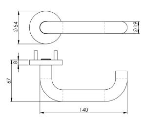
A substantial round bar return to door safety lever on a concealed fix bearing round rose. Grade 304 version. Concealed fix 2 part screw on rose. Certified to BS EN 1906 and BS EN 8300 to meet the needs of disabled people.
