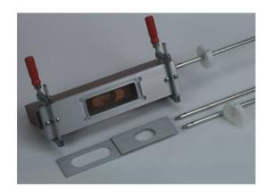
Fitting Jig for the 1129 & 1130 Ceam 3D concealed hinge.
