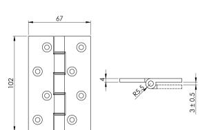
Solid brass hinges, polished and finished with a protective lacquer. Featuring non-rusting phosphor bronze washers for longevity. The Butt Hinge is often considered more appropriate in residential properties due to the size of the hinge knuckle being smaller and more discreet than the knuckle on ball bearing hinges. Suitable for standard internal residential doors a pair of hinges is adequate; however fitting 3 hinges per door has its advantages.
