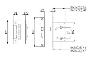
Contract Bathroom Lock with a wide range of options offering an excellent degree of choice. Square or Radius Forends, 65mm or 78mm sizes and 5 finishes. The Latch bolt has the Easi-T reverse function to save undoing the case so it can be reversed in seconds. Certified to BS EN 12209.
