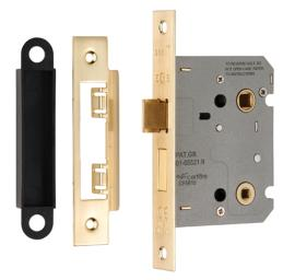
Contract Bathroom Lock with a wide range of options offering an excellent degree of choice. Square or Radius Forends, 65mm or 78mm sizes and 5 finishes. The Latch bolt has the Easi-T reverse function to save undoing the case so it can be reversed in seconds. Certified to BS EN 12209.
