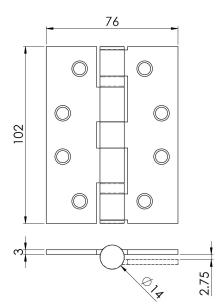
Grade 13 Ball Bearing Hinge, Square (Max Load 120kg). The most popular type of door hinge on the market today. These are a perfect choice for when you have doors of 40mm or 44mm, internal or external. They have a CE mark and are Certifire tested.
